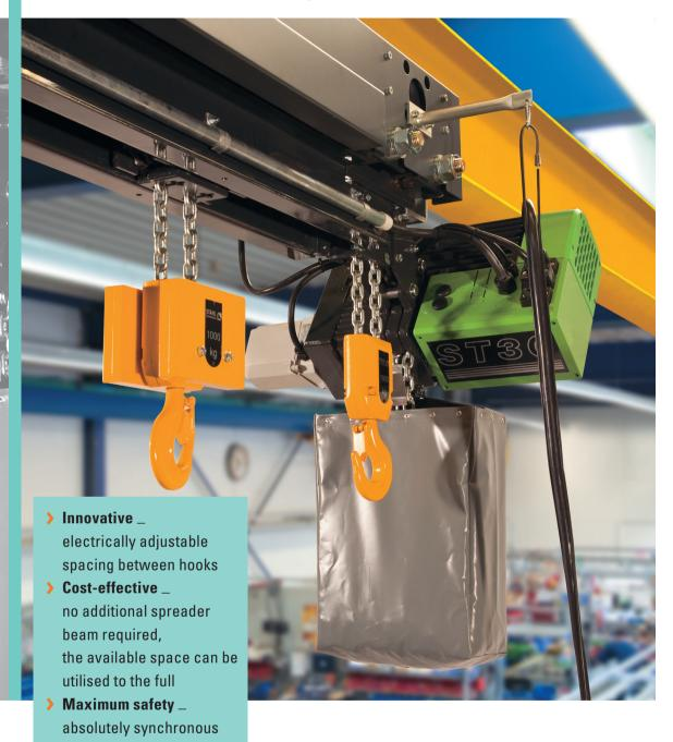
operation when transporting loads of different lengths, the load hooks cannot be displaced
