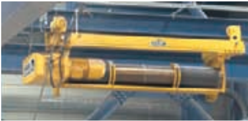
SH 6 wire rope hoist _ safe handling, true vertical lift thanks to two-rope design.
